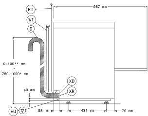
Drain ΕI Electrical inlet (power)
